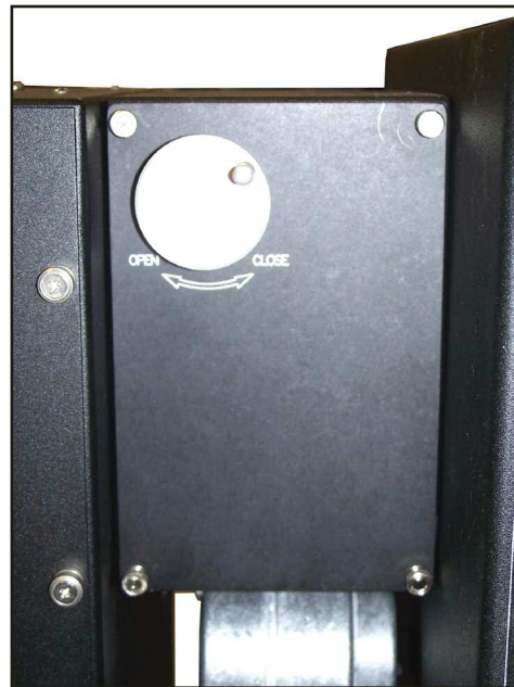
Partial Sun Attenuator module installed in Sol3A (6x6)
